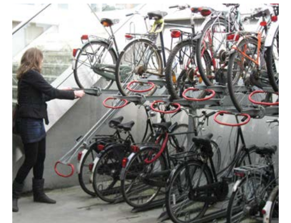
▲ Example of a two-tier bike rack system proposed in basement secure & sheltered long term bike parking
